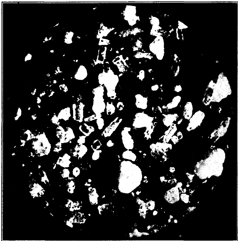
FIGURE 50. Commercial Sample of Tetryl (20 \times ). Material crystallized in this form pours easily and may be made into pellets by machinery.
